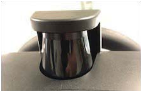
Figure 94: Upper LIDAR sensor
