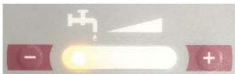
Figure 41: Set the solution flow control
